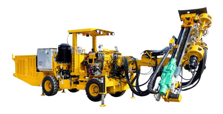
RAPTOR 44-2R is an electrohydraulic rig for long hole drilling, its hydraulic boom has automatic parallelism, equipped with two rotary actuators allow drilling very close to both walls of the section of the mine.
