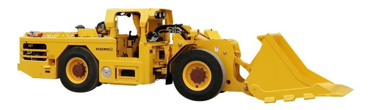
The SFL 35, is specially designed for underground mining works in narrow section. With a width of 1.40 m and tramming capacity of 3.5 tones, is ideal to raise your productivity without the need of increasing your gallery sections.
