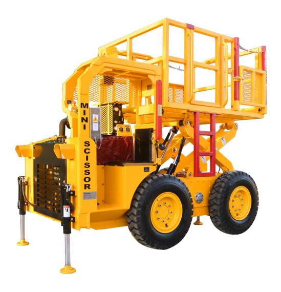
The SURI 22 MINI SCISSOR LIFT, is specially designed for underground mining works in narrow section. With a width of 1.60 m, height of 2.16 m and loading capacity of 1.5 tons, the SURI 22 fits 2.5 x 2.5 m.
