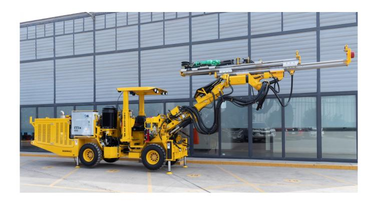
TROIDON 44 XP is a front face drilling rig of 1.30 m width recommended for small sections from 2.50 m x 2.50 m to 4.50 m x 4.50 m.
